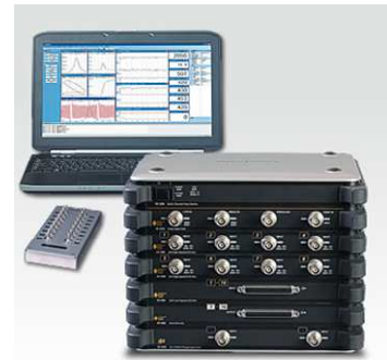
Fig. 21 Combustion analysis device (Ono sokki: DS3000)
