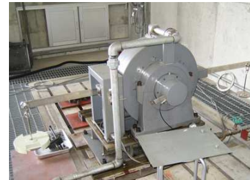
Fig. 4 Appearance of eddy current engine dynamometer
