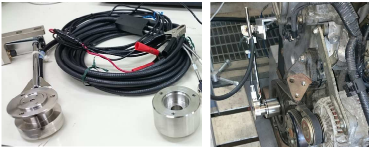
Fig. 20 Crank angle position detector (Ono sokki: CP-5900 and CA-6000A)
