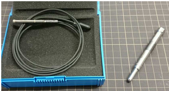
Fig. 18 Pressure sensor (Kistler: Type6056A) and glow plug adapter
