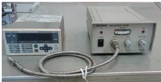
Fig. 26 Non-contact type rotation detector and advanced tachometer (Ono sokki : FS-540, FG-1200 and FT-1500)
