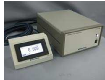
Fig. 14 Laminar flow computer (Sokken LFC-200)
