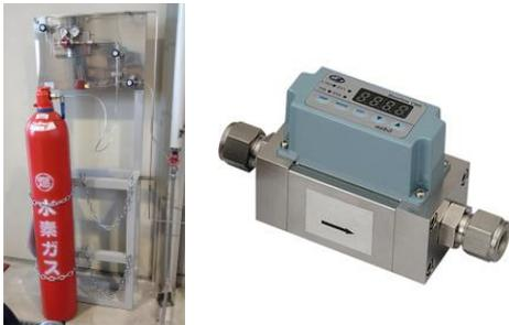
Fig. 6 H<sub>2</sub> supply device and flowmeter for H<sub>2</sub>
